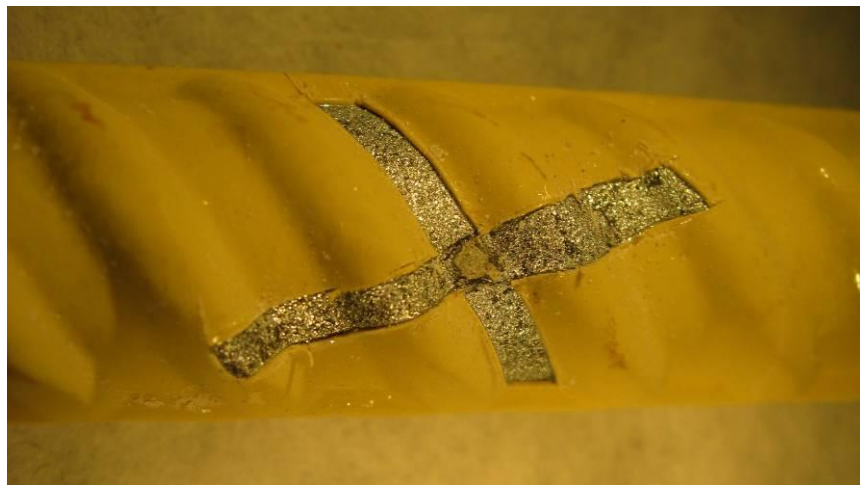
Figure 12: Specimen Subjected to the Disbondment Measurement Procedure. Specimen was polarized to -500 mV with no-chloride exposure.
