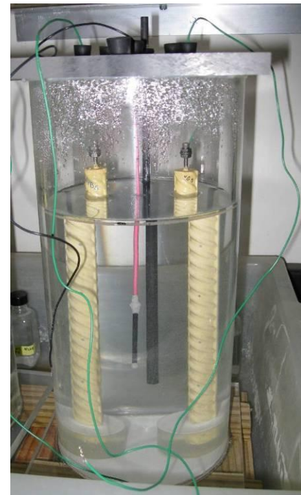
Figure 17: Supplemental OCP No-chloride Exposure Test Cell.
