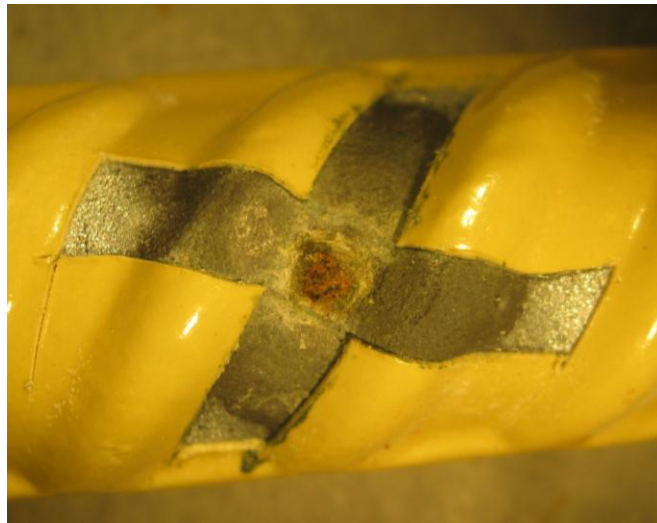
Figure 34: Discolored Area Around Defect Observed for the +100 mV Chloride Exposure Specimens. Specimen YG3.
