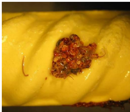
Figure 19: Solid Corrosion Product that Developed on +100 mV Chloride Exposure Specimens. Specimen YG3
